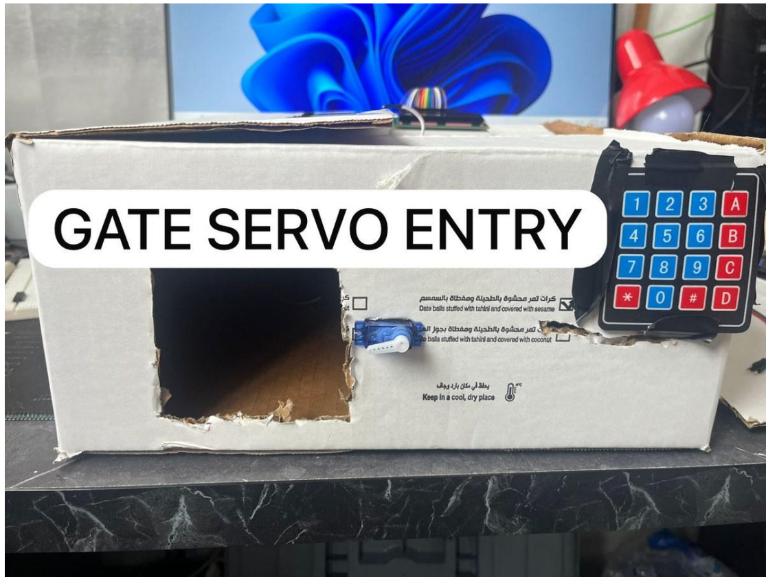
Fig. 12. Gate servo entry and keypad.
